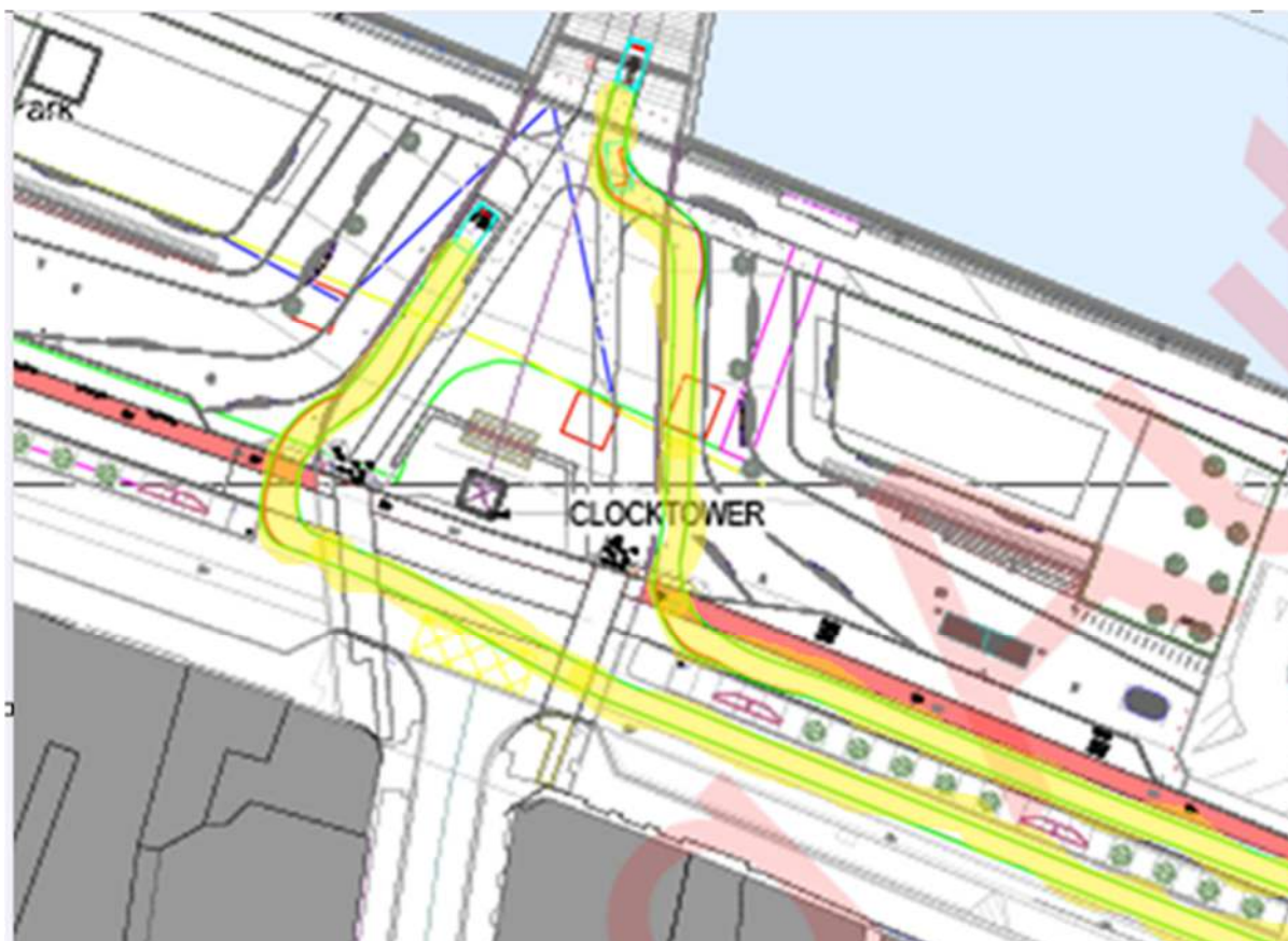
Figure 17 Swept Path Analysis for a bus from South Plaza to Meagher's Quay - - the yellow lines show the path of a small shuttle bus
